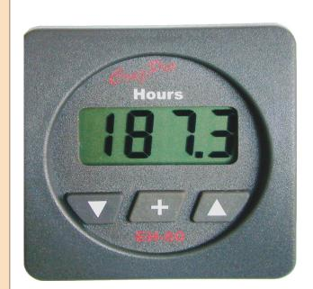
The **EH60** is a full featured Engine Hours and Elapsed Trip Time gauge which displays total engine hours and elapsed trip time from 000.0 hours to 9999 hours. A built-in engine hours countdown alarm can be set to warn you to perform needed maintenance such as changing the engine oil or oil filters. When activated the builtin alarm will sound and the display will flash.
