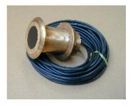
The CruzPro DSP (Digital Signal Processing) Active Transducers output NMEA 0183 serial data of depth and water temperature. Numerous models suit most applications requiring NMEA \$SDDPT, \$SDDBT and \$SDMTW depth/temperature data.
